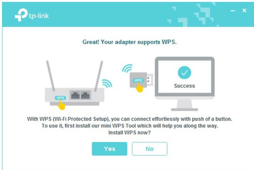
5. When the following screen appears, the WPS Tool has been installed successfully. You can enjoy connecting to your Wi-Fi with the push of the WPS button.
